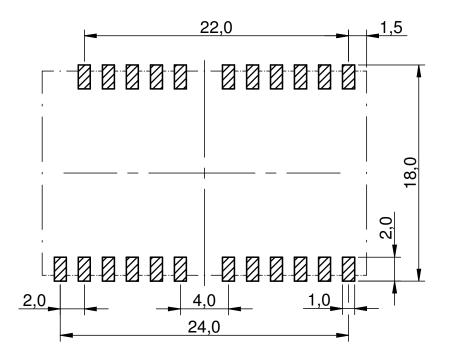
Figure 12: Footprint and dimensions [mm]
