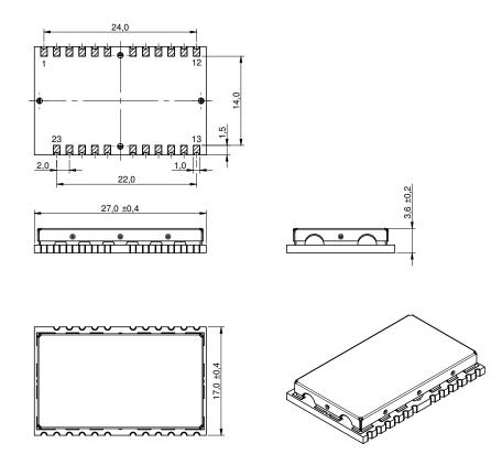
Figure 11: Module dimensions [mm]
