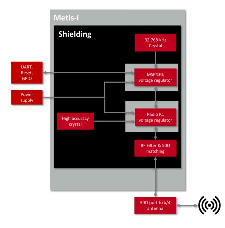
Figure 1: Block diagram of the Metis-I module
